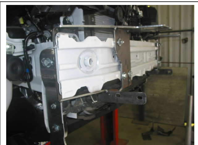
Figure 5: Install ECB steel mounting brackets onto bumper support
