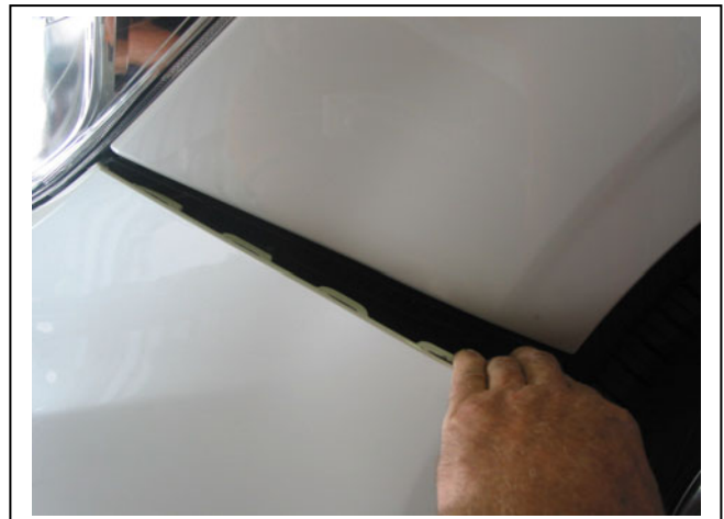
Figure 2: Unclip bumper from guard and light
