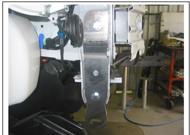
Figure 4: Install tow hook to passengers side, use 40 x 6 washer to rear of lower hole
